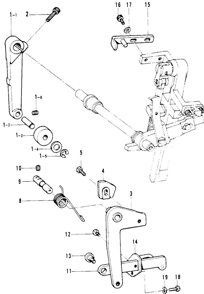
**J. Tension pulley mechanism**
